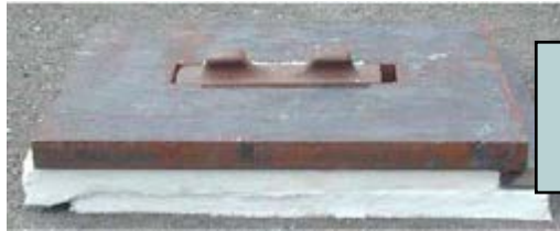
Liner plate and based showing fibre insulation
