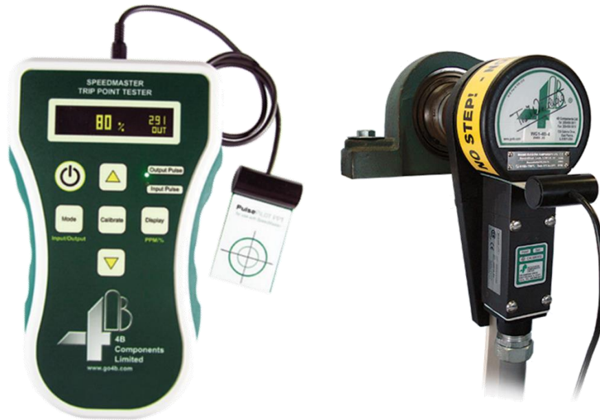
Figure 43: Speed sensor tester (left) and connected to sensor in universal shaft mount. (Photo courtesy of 4B Components, Ltd.)
