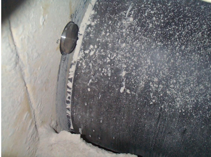
Figure 21: Interior view of belt conveyor head with misalignment sensor monitoring both belt and pulley. (Photograph courtesy of 4B Components, Ltd)
