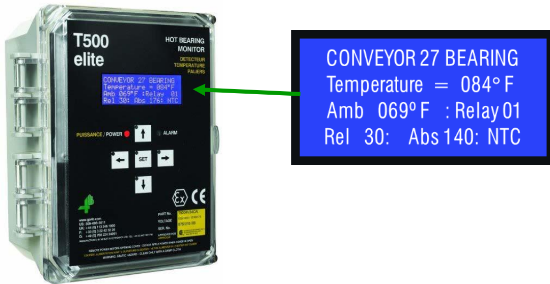
Figure 22: Continuous bearing temperature-monitoring system. (Photograph courtesy of 4B Components, Ltd)
