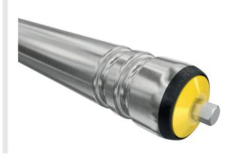
Grooves are running grooves that can be placed in steel tubes. They are used to guide round belts. When using the corresponding round belt, they are below the roller surface and, as such, do not contact the conveying good.
