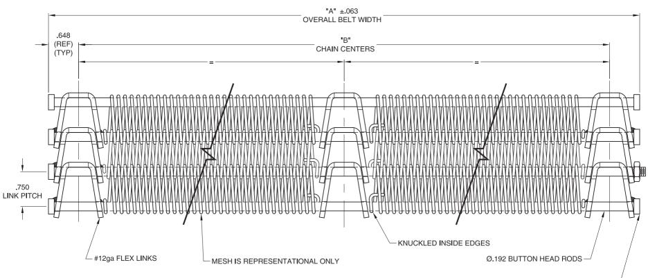
TYPICAL BUTTONHEAD ON BOTH ENDS OF ALL RODS EXCEPT CONNECTING RODS. ----
