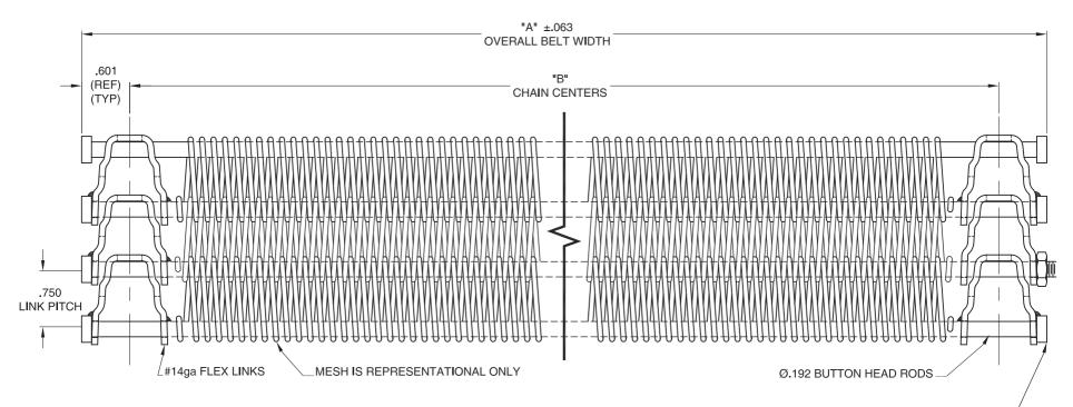
TYPICAL BUTTONHEAD ON BOTH ENDS OF ALL RODS EXCEPT CONNECTING – RODS.
