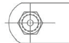
Pin Style #5 Hug Locknut Multiple grease fittings options available
