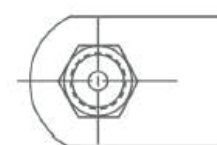
Pin Style #5 Hug Locknut Multiple grease fittings options available
