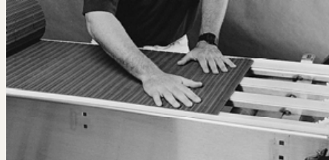
Figure 8: Feed belt from drive end
